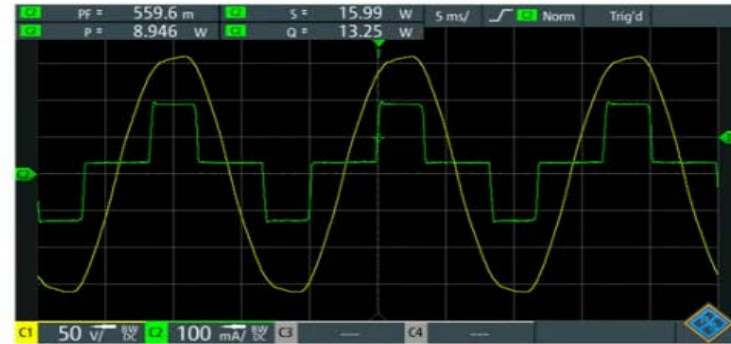
LED bulb (60W equivalent) lower PF (0.56), lower active power (9 W)
